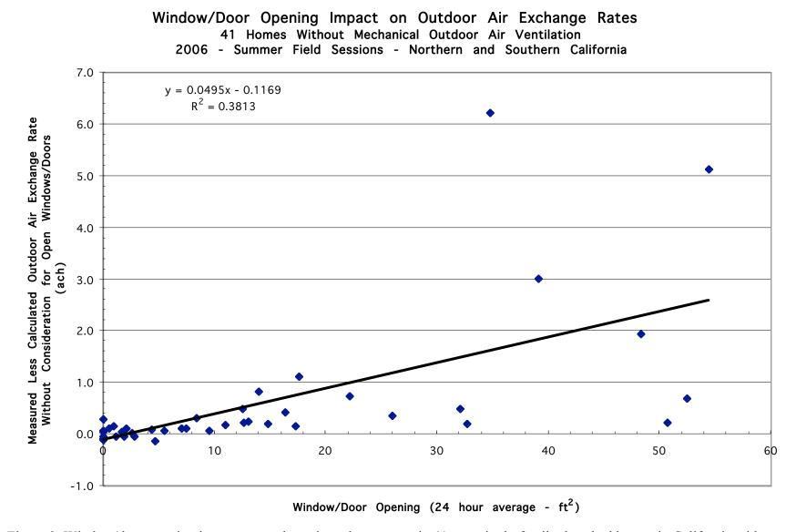
Figure 3. Window/door opening impact on outdoor air exchange rates in 41 new single-family detached homes in California without mechanical outdoor air ventilation.
