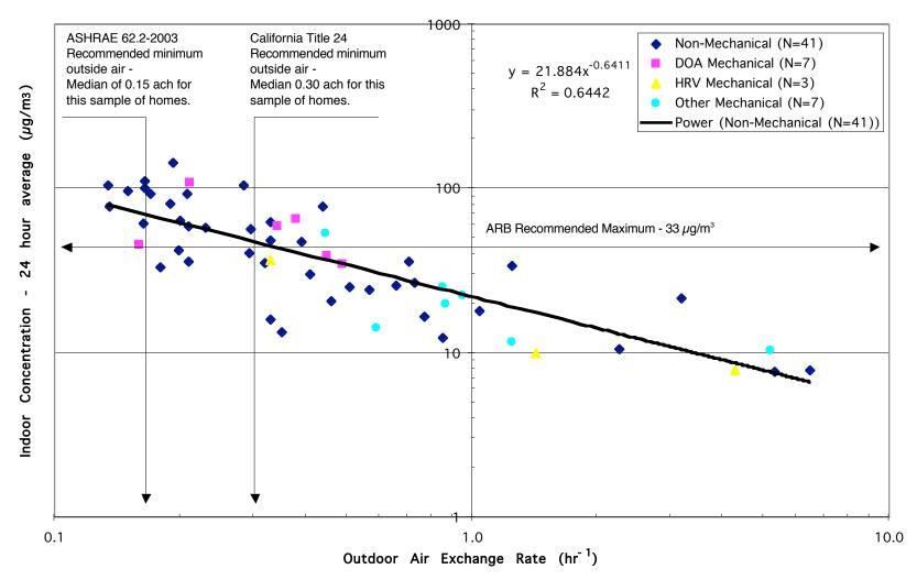
Figure 4. Indoor formaldehyde concentrations and outdoor air exchange rates in new single-family detached homes in California, 41 homes without and 17 homes with mechanical outdoor air ventilation. Power curve fit of non-mechanically ventilated home data.
