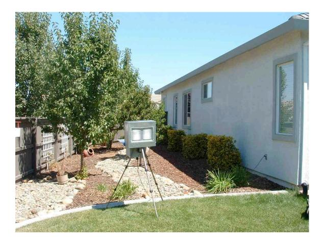
Figure 2. Outdoor air sampler for formaldehyde, VOC's, PM<sub>2.5</sub>, NO<sub>2</sub>, CO, CO<sub>2</sub>, temperature, and relative humidity, with outdoor radiation/rain shield.
