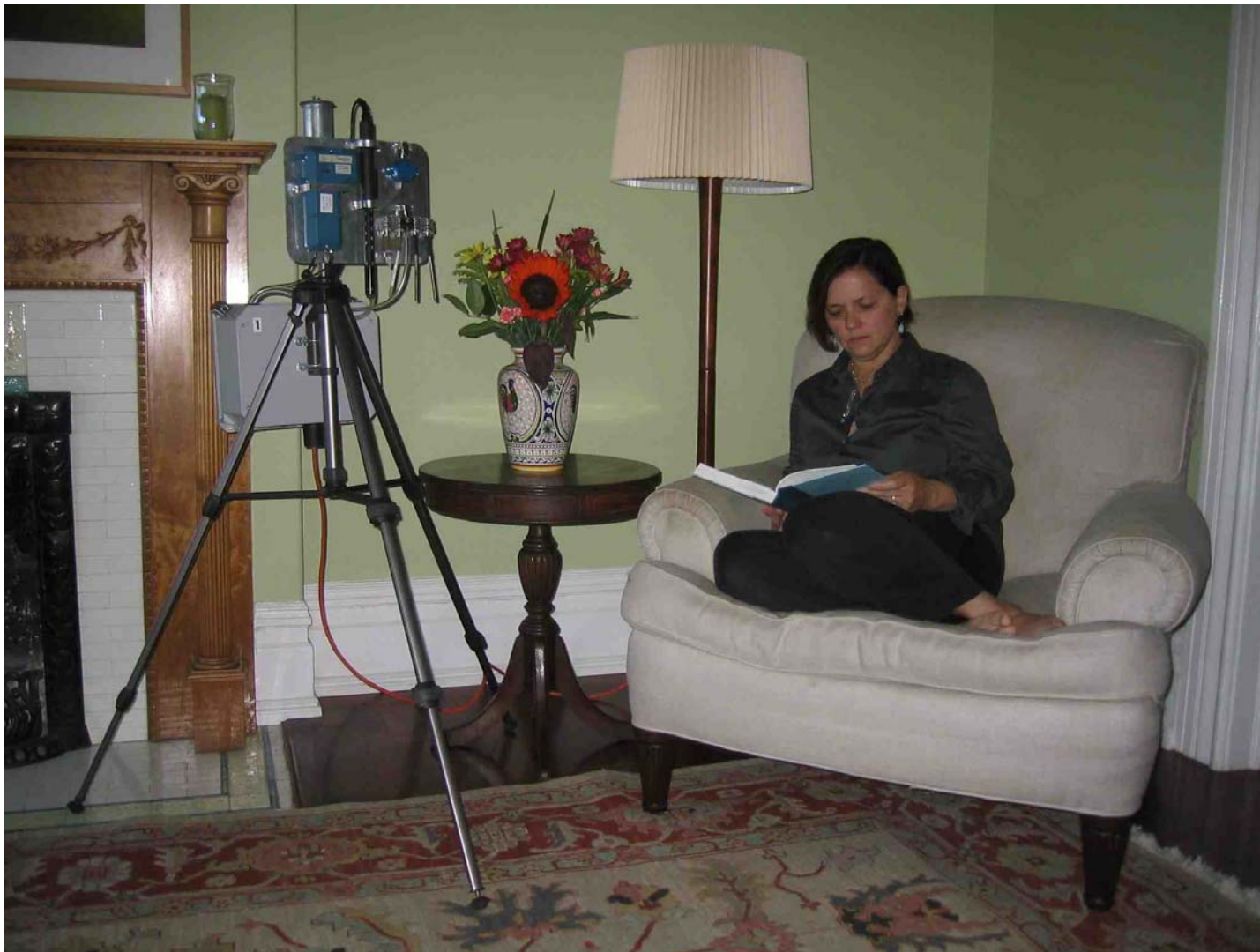
Figure 1. Quiet indoor air sampler for formaldehyde, VOCs, PM 2.5 , NO 2 , CO, CO 2 , temperature, and relative humidity, typically installed in a home living/dining room area for a 22–26 hour sampling period.
