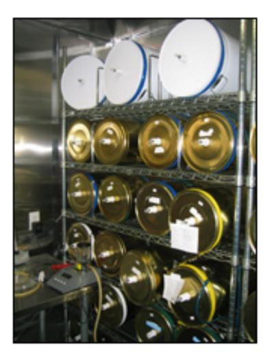
Indoor Environmental Engineering provides on-site measurements of the chemical emission rates from installed flooring and other indoor finishes.
