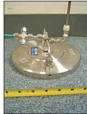
Picture of the FLEC emission cell that can be used to measure contaminant emission rates of building materials onsite after materials have been installed.
