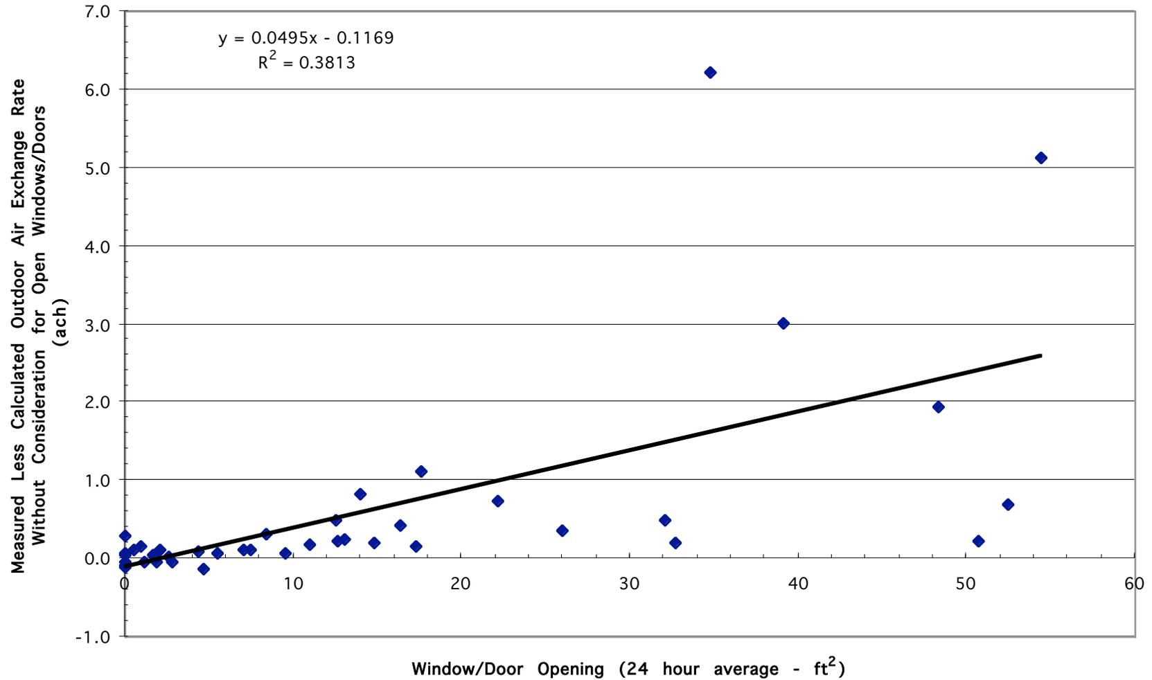
Figure 3. Window/door opening impact on outdoor air exchange rates in 41 new single-family detached homes in California without mechanical outdoor air ventilation.
