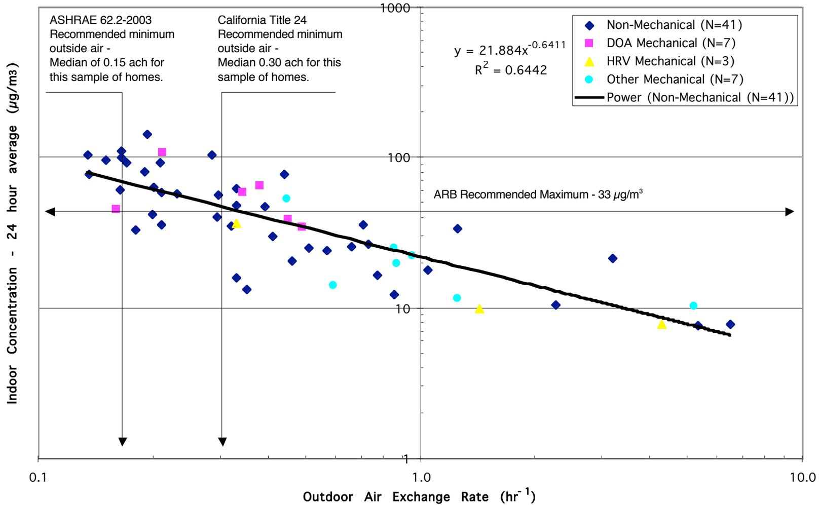
Figure 4. Indoor formaldehyde concentrations and outdoor air exchange rates in new single-family detached homes in California, 41 homes without and 17 homes with mechanical outdoor air ventilation. Power curve fit of non-mechanically ventilated home data.
