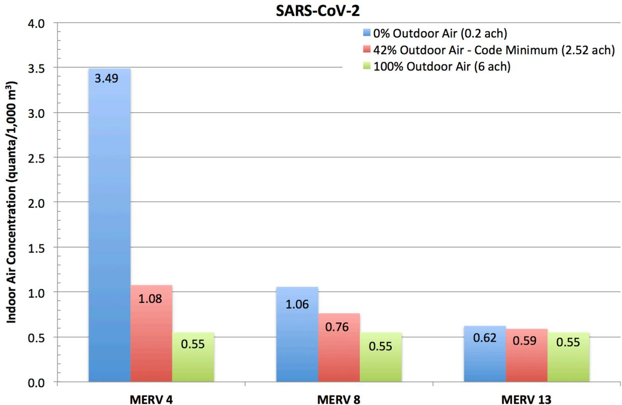
Figure 2. Modeled indoor SARS-CoV-2 concentrations for three ventilation and three air filtration scenarios.
