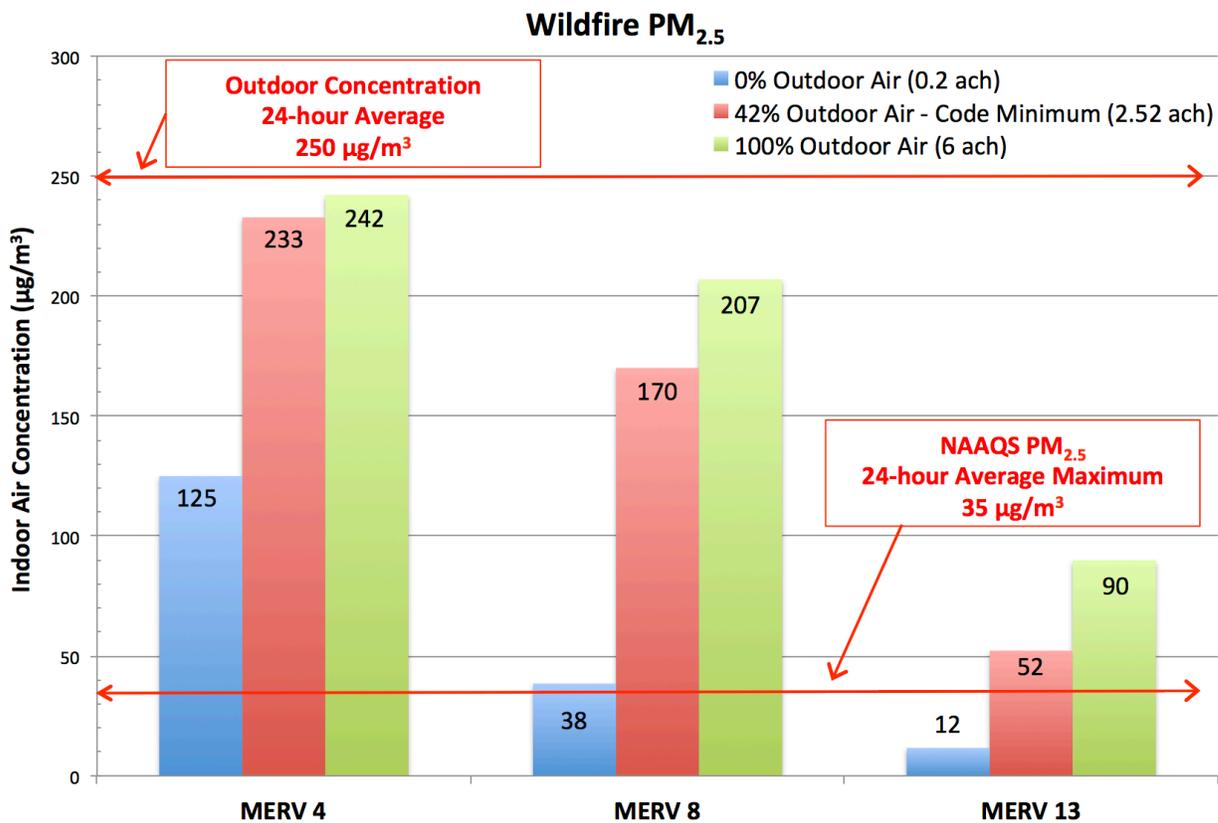
Figure 1. Modeled indoor wildfire  $PM_{2.5}$  concentrations for three ventilation and three air filtration scenarios.
